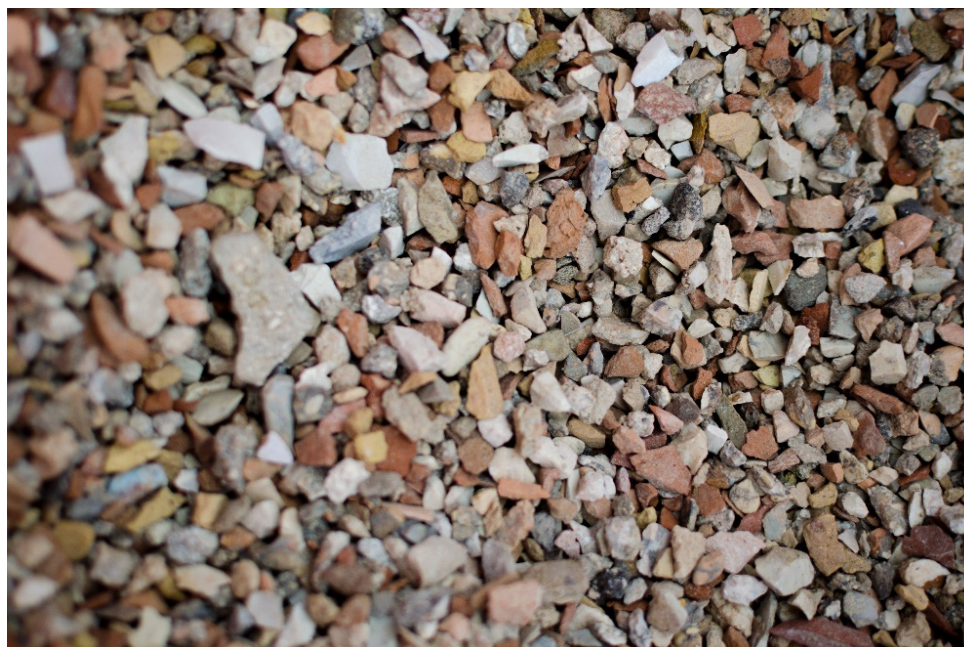
Figure 4. Recycled aggregates generated from the rubble of the 2016 earthquake in Central Italy.
