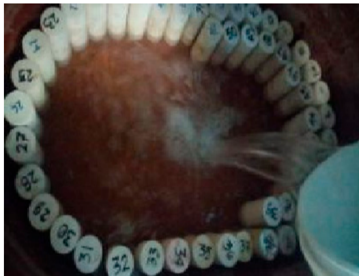
Figure 6. Procedure for determining the water content of Rock Samples.
