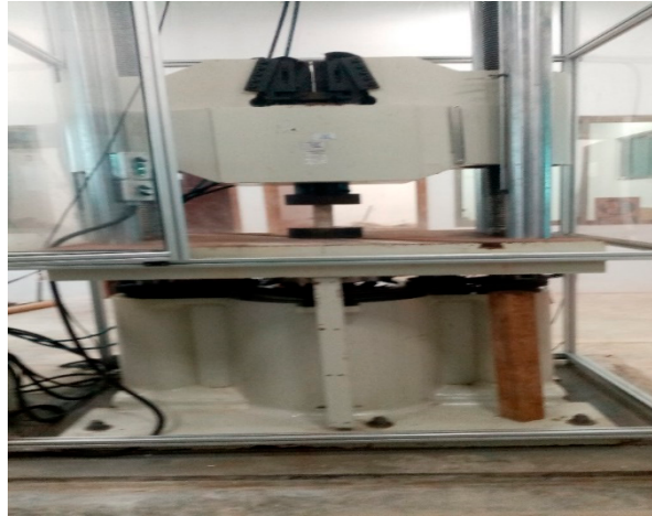
Figure 4. The specimen is positioned at the center of the compression platens in the Universal Testing Machine.
