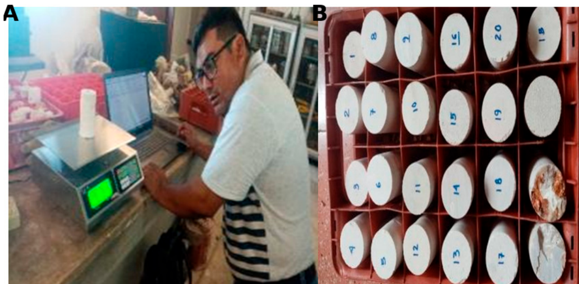
Figure 7. Real density determination of rock specimens: (A) measurement of specimen mass; (B) determination of specimen volume.
