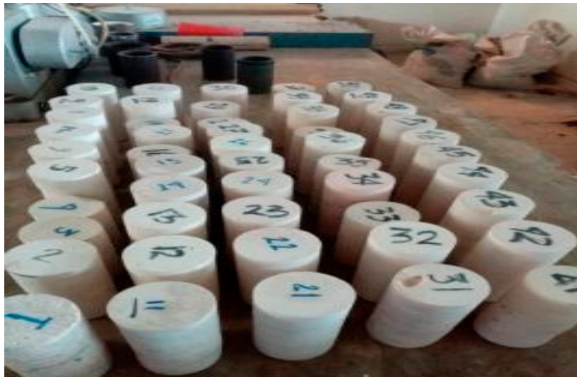
Figure 3. Array of straight, circular, cylindrical rock specimens prepared for mechanical testing.
