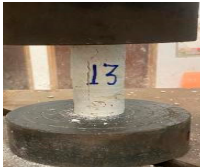
Figure 5. Compression Test in Progress.
