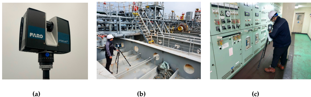
Figure 2. High-precision 3D laser scanning infrastructure and its on-site application: (a) FARO Focus M70 terrestrial laser scanner; (b,c) Data acquisition and spatial surveying within complex maritime structures.
