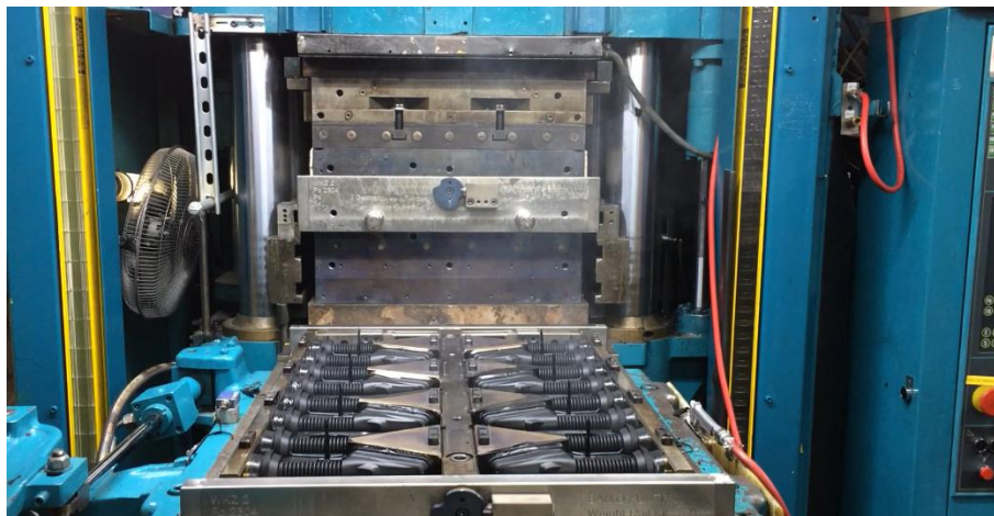
Figure 12. – Testing of an injection-moulded door grommet for automotive applications.
