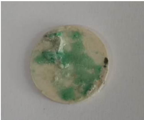
Figure 6. Showing Complexation of \text{Ni}^{2+} on the surface of the S2 membrane.
