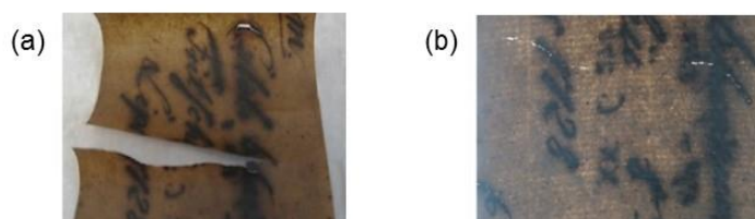
Figure 7. Damaged sample: (a) before and (b) after mechanical stabilization with nanofibrillated cellulose and chemical stabilization with calcium phytate/calcium hydrogen carbonate (Reproduced with permission from Völkel et al. Copyright © 2020, Springer).
