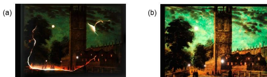
Figure 6. One viewing slide from the French Museum of Cinema under transmitted light: (a) before and (b) after treatment with microfibrillated cellulose film (Reproduced with permission from Dreyfuss-Deseigne. Copyright © 2017, Taylor & Francis).
