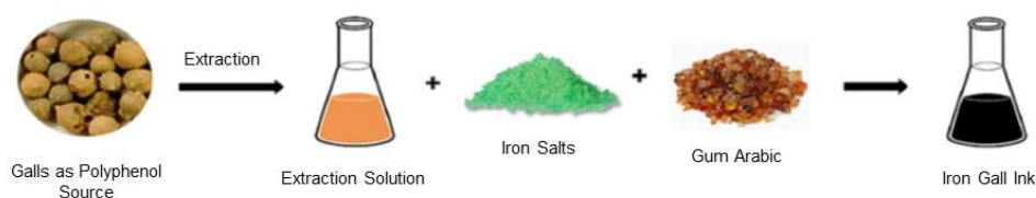
Figure 2. Main steps involved in the preparation of iron gall ink (Reproduced with permission from Díaz Hidalgo et al. Copyright © 2018, Springer).
