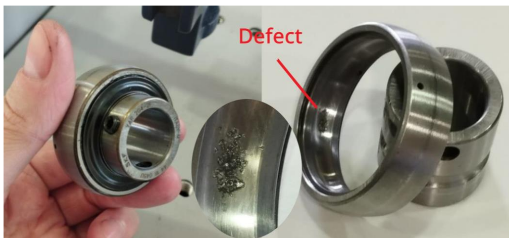
Figure 3. Detailed view of the damaged bearing: (left) assembled SKF YAR 204 2F unit; (right) disassembled outer race highlighting the localized defect (approx. 5 x 3 mm); (center) magnified detail of the spalling area.
