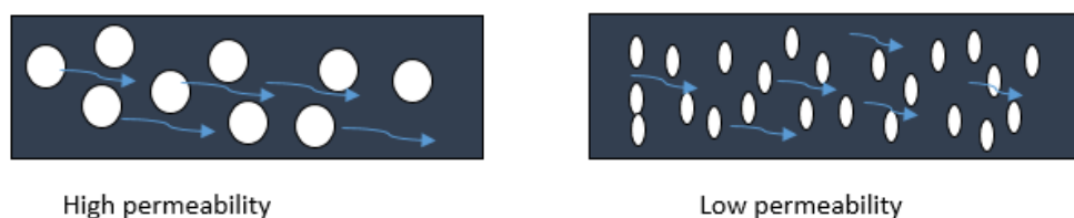
Figure 6. shows the difference between high and low permeability.
