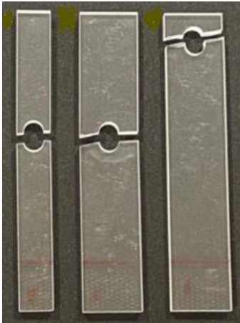
Figure 5. Specimen fracture with 8 mm pin: left) Specimen #1, center) Specimen #2, and right) Specimen #3.
