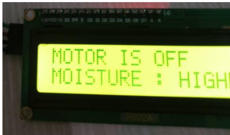
Figure 14. LCD Output When Moisture is High.
