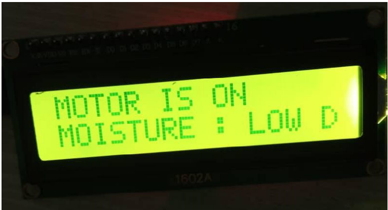
Figure 12. LCD Output When Moisture is Low.
