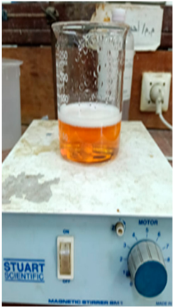
Figure 6. Preparation of selenium nanoparticles by reduction with Ascorbic acid.
