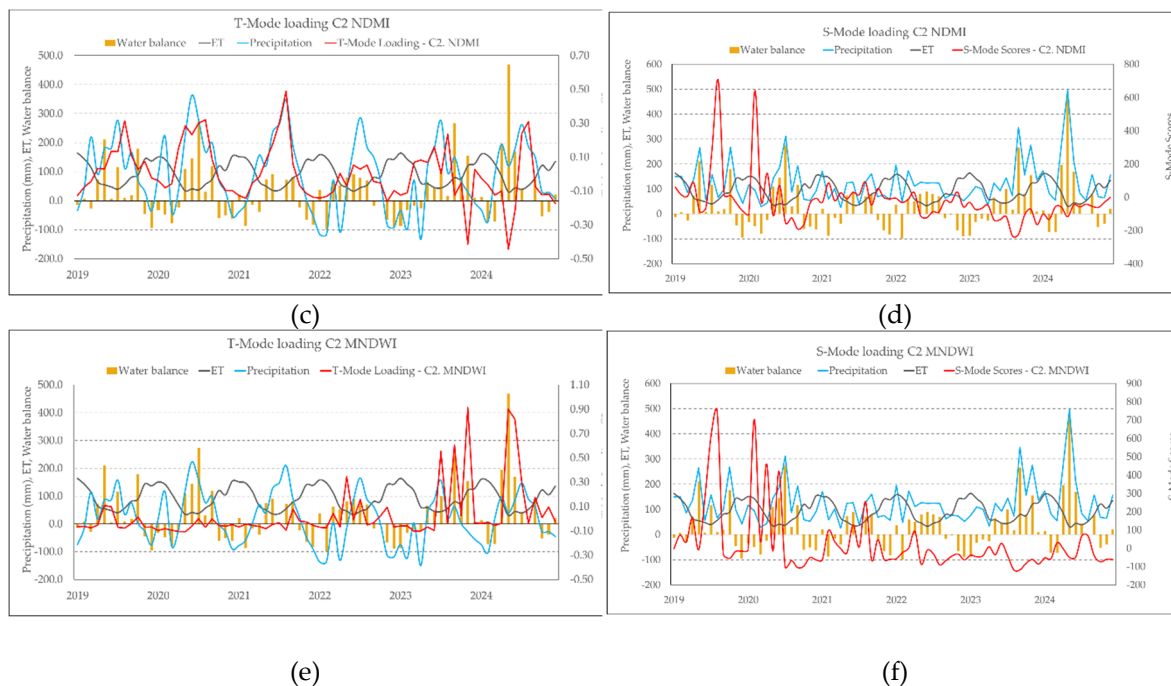
Figure 8. Estimated values of precipitation, evapotranspiration, and water balance from 2019 to 2024. C2 loadings and scores by hydrogeomorphological attribute, presented for both T-Mode and S-Mode analyses. NDVI (a,b), NDMI (c,d), MNDWI (e,f).
