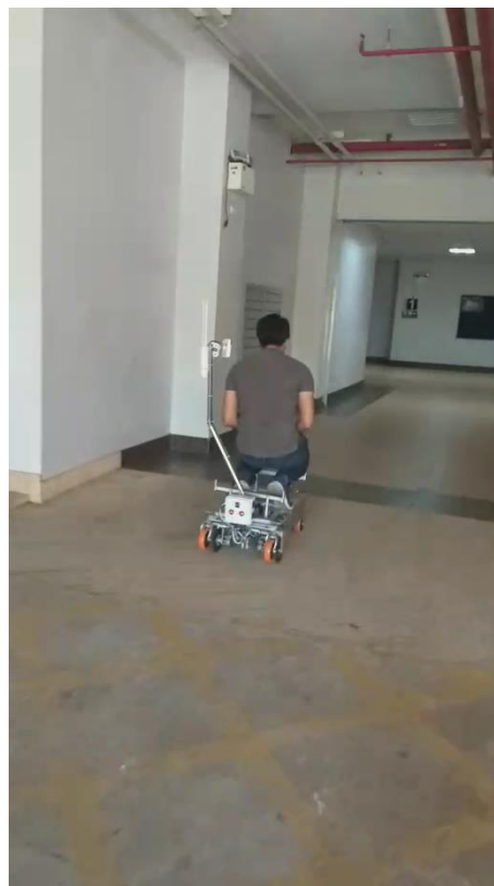
Figure 7. The test of the delivery function when loaded an 85 kg man
