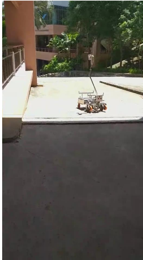
Figure 8. The test of the driving system when operating on level ground, measuring 30° to 45° in declination angle
