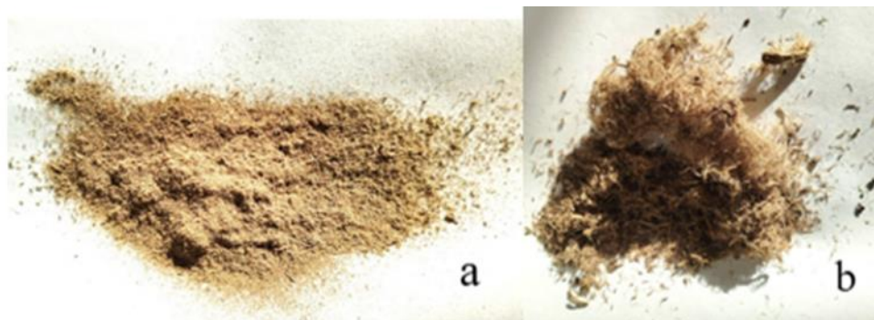
Figure 4. Industrial waste licorice root, pulverized after the grinding process (a), industrial waste licorice root, broken after the segmentation process (b).
