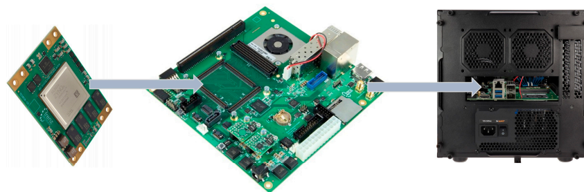
Figure 5. Main components of the Edge Computing prototype. Left: Module containing the SoPC component and memory chips. Middle: The ITX base board provides one module place. Right: Integration into a standard housing. (Collage of images from Trenz with their kind permission)
