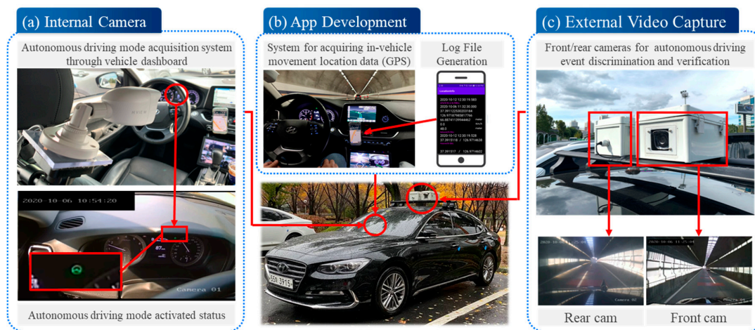
Figure 1. Devices installed for data collection: (a) an in-vehicle camera used to capture the activation status of the LKAS; (b) a mobile application installed to record the GPS coordinates and reasons for LKAS disengagement; (c) external cameras mounted to capture front and rear views of the vehicle.
