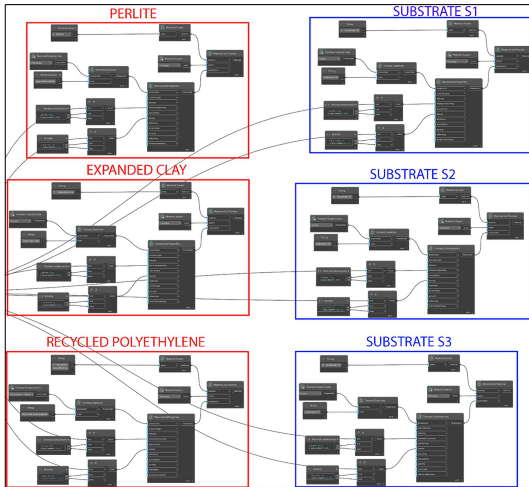
Figure 4. Material creation for drainage layers (in red) and substrates (in blue).
