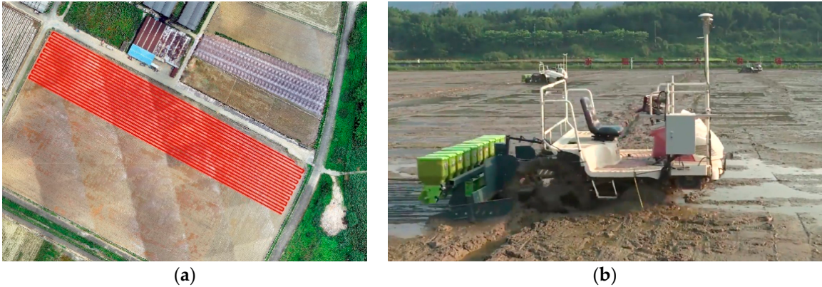
Figure 10. Planned working path and field site for unmanned direct seeding machine: (a) Planned working path; (b) Field site.
