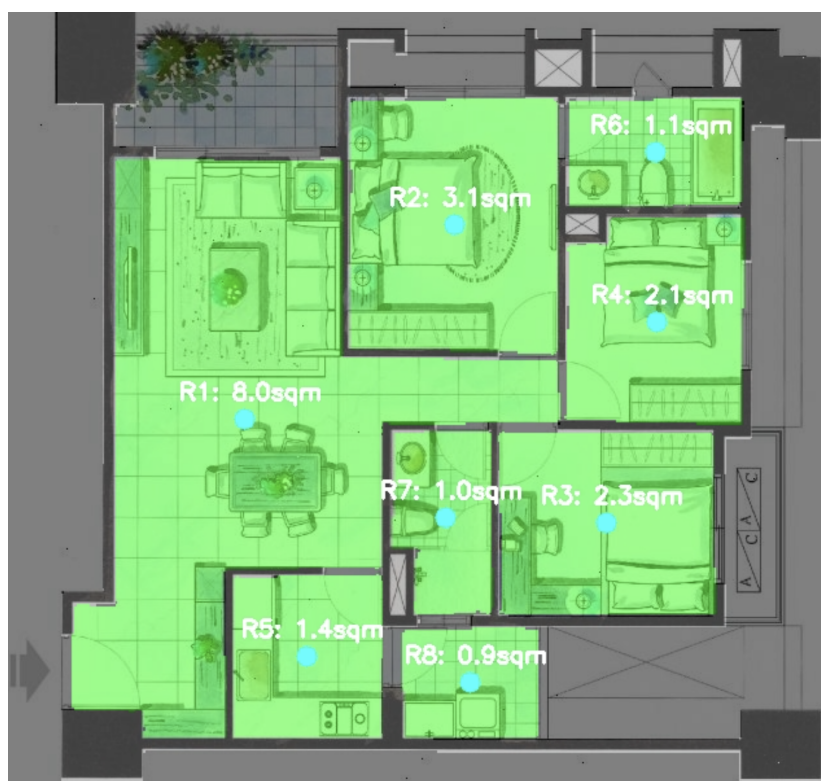
Figure 6. U-Net segmentation masks (Green: Room, Gray: Wall), automatically generates an area calculation report alongside furniture statistics.
