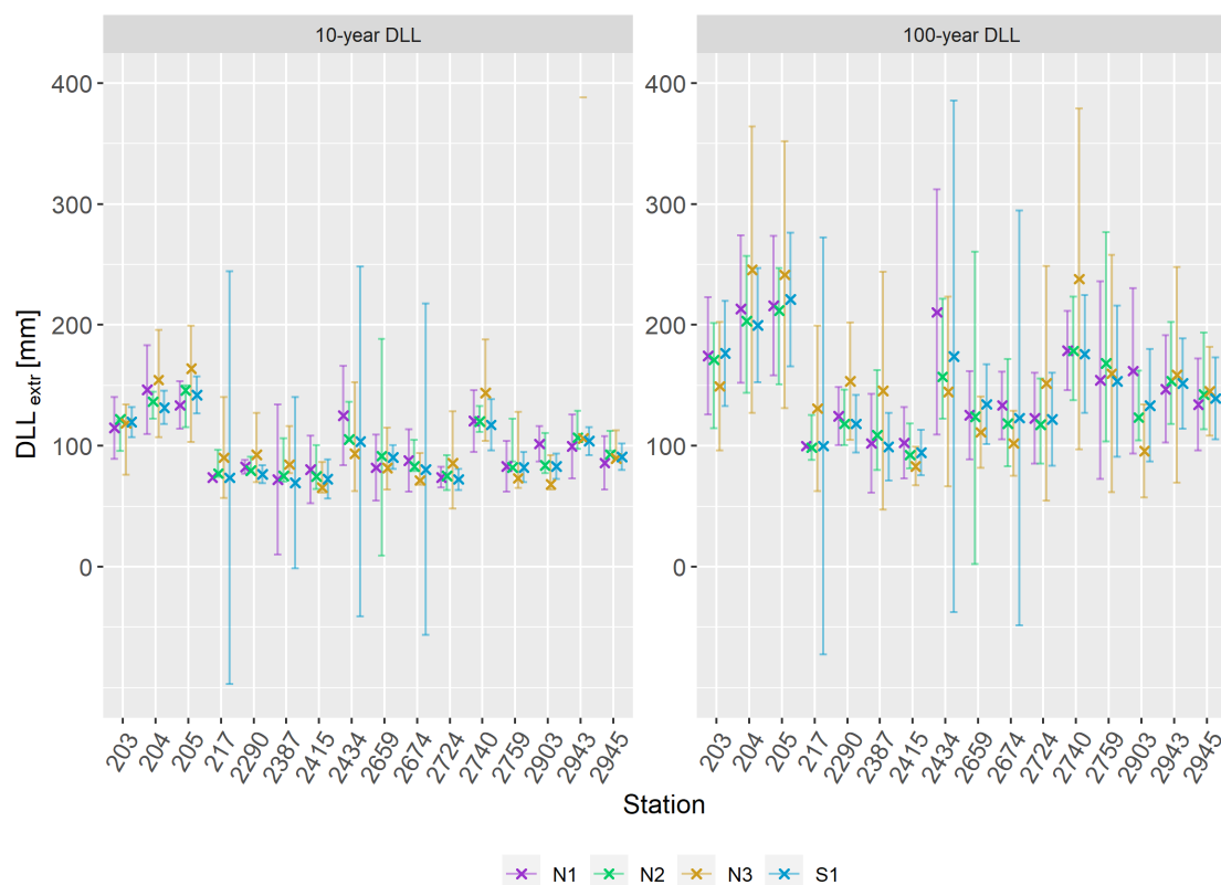
Figure 8. 100-year and 10-year DLL_{extr} obtained from extrapolated statistical models (2071–2100) with parameter estimation method MLE.
