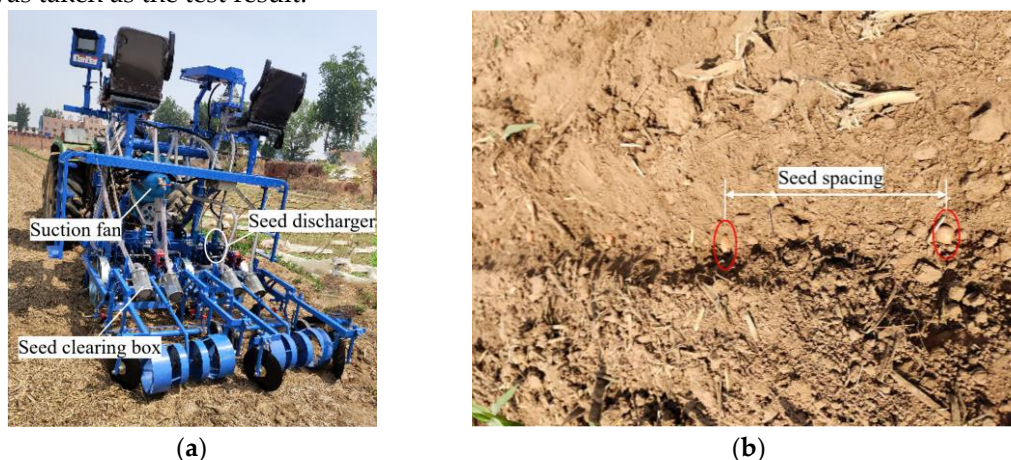
Figure 23. (a) Installation position of the seed discharger on the planter; (b) The spacing between seeds.
