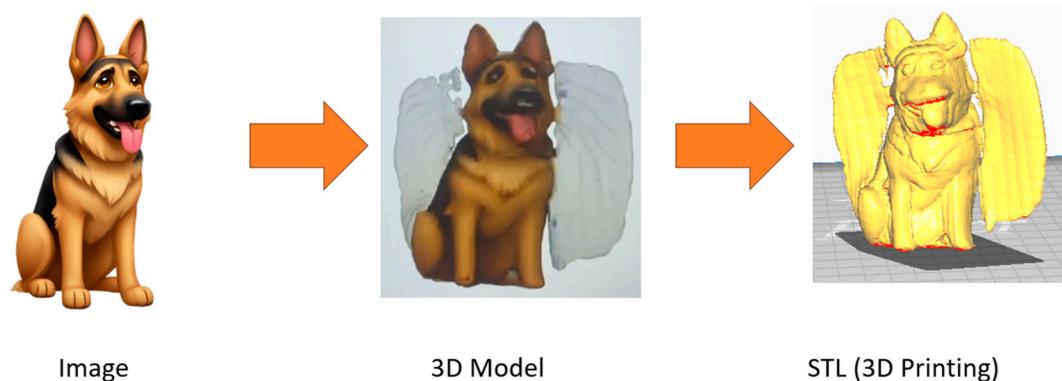
Figure 10. Conversion of a static 2D image to a 3D printable model with software pipeline.
