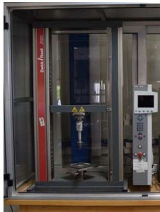
Figure 4. Zwick/Roell Z020 Universal testing machine.
