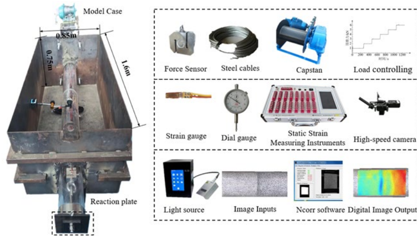
Figure 3. Indoor deflection test system for pipe jacking.
