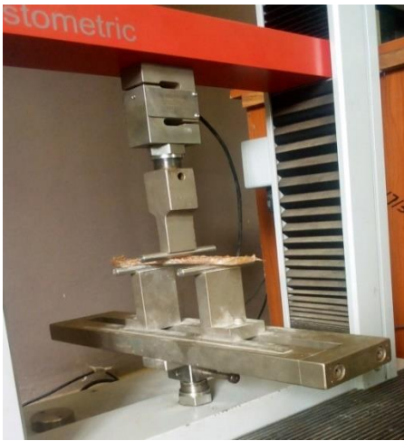
Figure 2.4. Flexural test setup.
