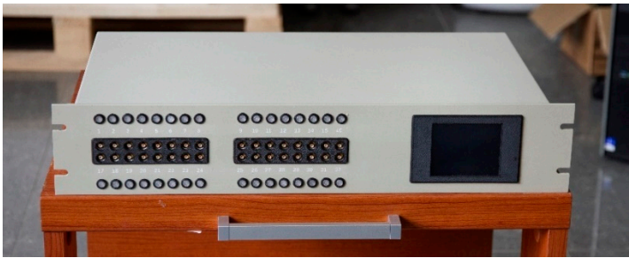
Figure 7. An electrical tomograph for measurements in electrical tomography
