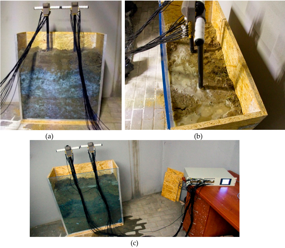
Figure 14. Laboratory model with one multi-sensor electrode: (a) front view, (b) top view, (c) during electrical tomography measurements
