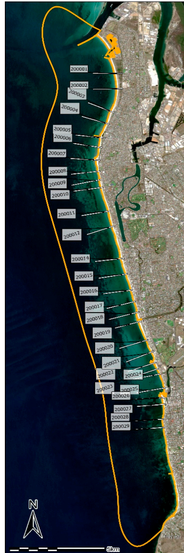
Figure 2. The spatial distribution of cross-shore profiles extending 1.5km seaward at 1km intervals. Profiles are numbered from 200001 in the north to 200029 in the south.
