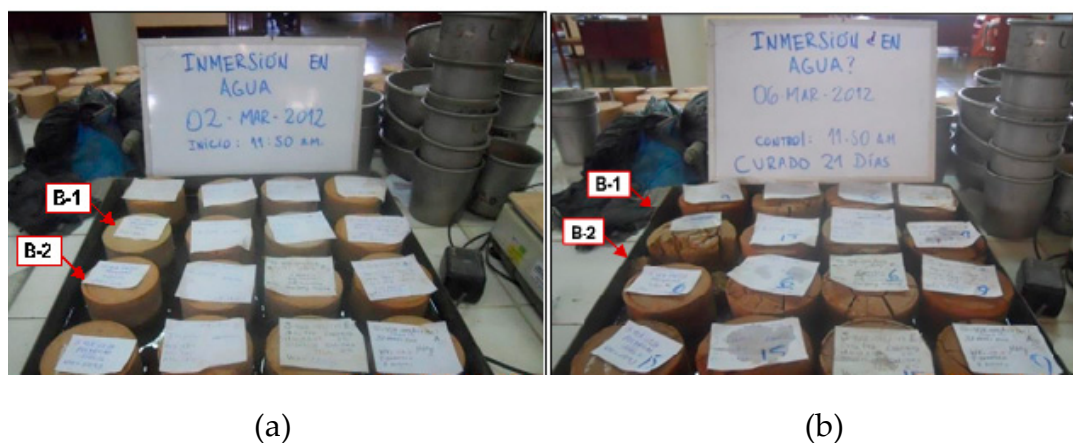
Figure 1. Stabilization Suitability of Clay Samples (a) Comparison of clay samples B-1 and B-2 after immersion in water, highlighting differences in stabilization suitability. Sample B-1, labeled in red, shows characteristics unsuitable for stabilization. (b) Detailed view of the clay samples post-immersion, with sample B-2, labeled in white, demonstrating favorable characteristics for stabilization.
