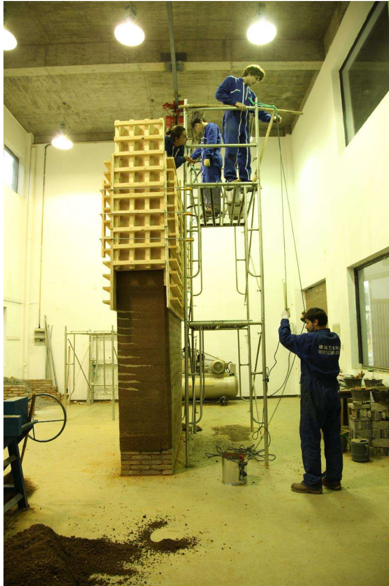
Figure 2. Construction of the first experimental earth wall at the Sustainable Construction Laboratory of China Academy of Art(©Chaochao Wei).
