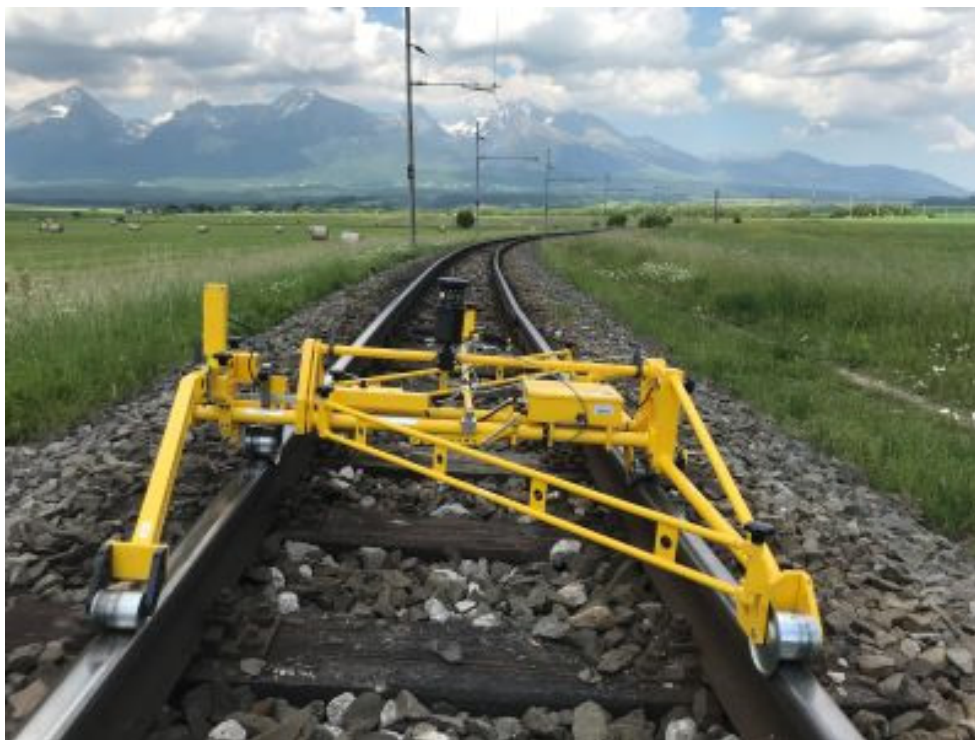
Figure 1. Digital mobil system KRAB™-Light with mounted reflector of robotic total station. Source: Comprehensive diagnostics of Tatra Electric Railway.
