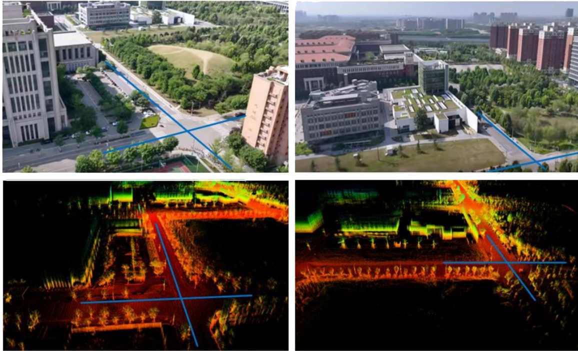
Figure 6. 3D mapping results of the UAV using the proposed algorithm.
