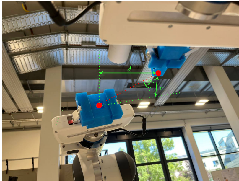
Figure 3. Quantities describing the geometric relationship between peg and hole.
