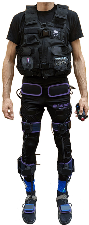
Figure 2. Components of the NeuroSkin® system. The textile-based system includes embedded dry electrodes targeting key lower-limb muscle groups, inertial and force sensors for gait monitoring, an AI-driven gait phase detector, a programmable electrical stimulator, and therapist-facing software for session management.
