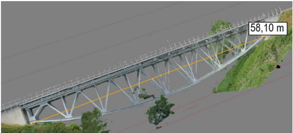
Figure 22. Agisoft 3D model measurement of the bridge span.
