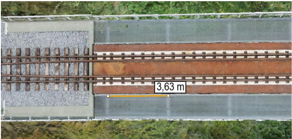
Figure 23. Agisoft 3D model measurement of the crossbeams spacing.
