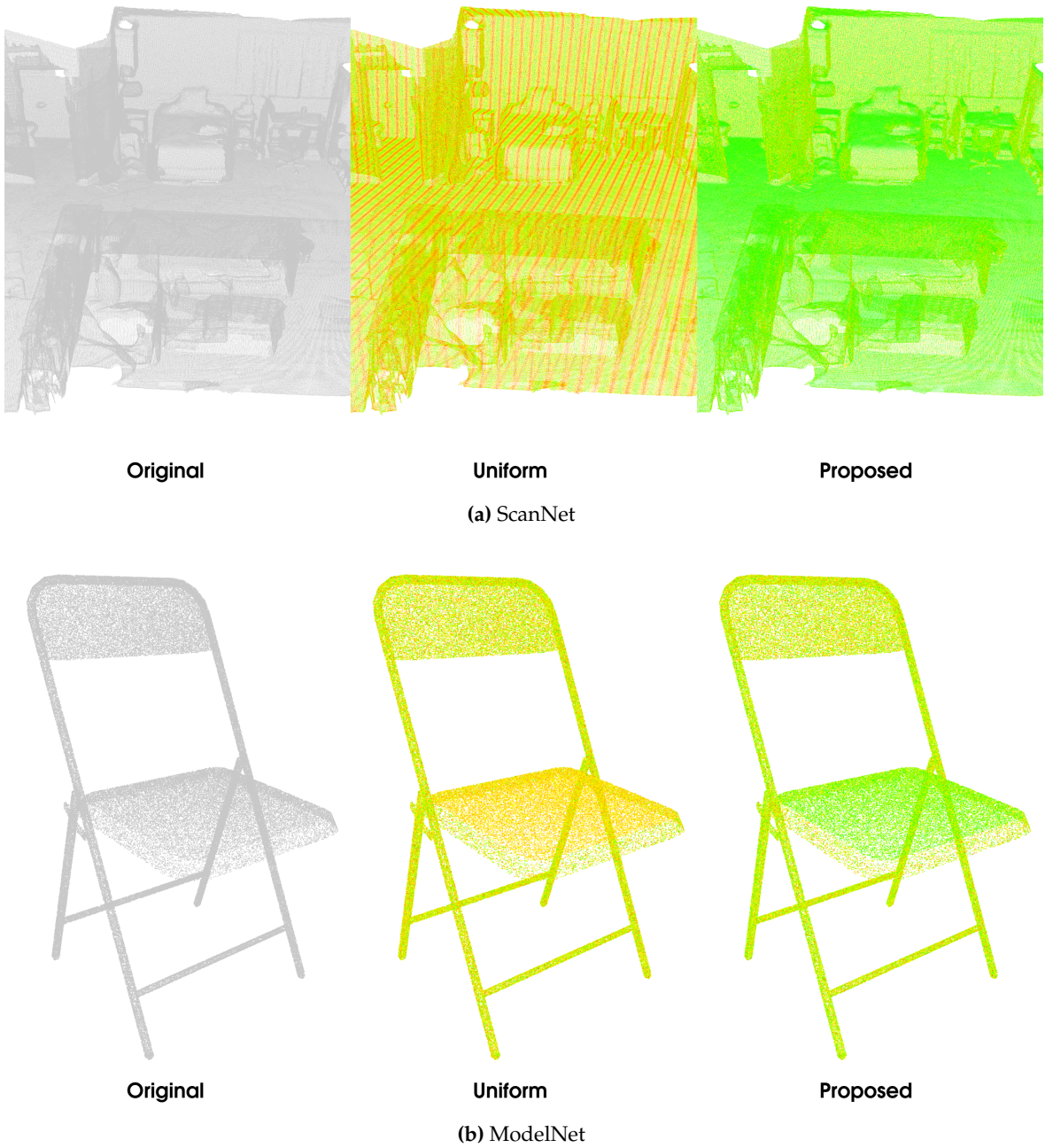
Figure 4. A qualitative comparison of uniform voxelisation and the proposed non-uniform voxelisation on a sample from the ScanNet 4a and ModelNet 4b datasets. Each point is coloured from red to green based on the Euclidian coding error (D1) for that point, the colour scale is shared between the methods.
