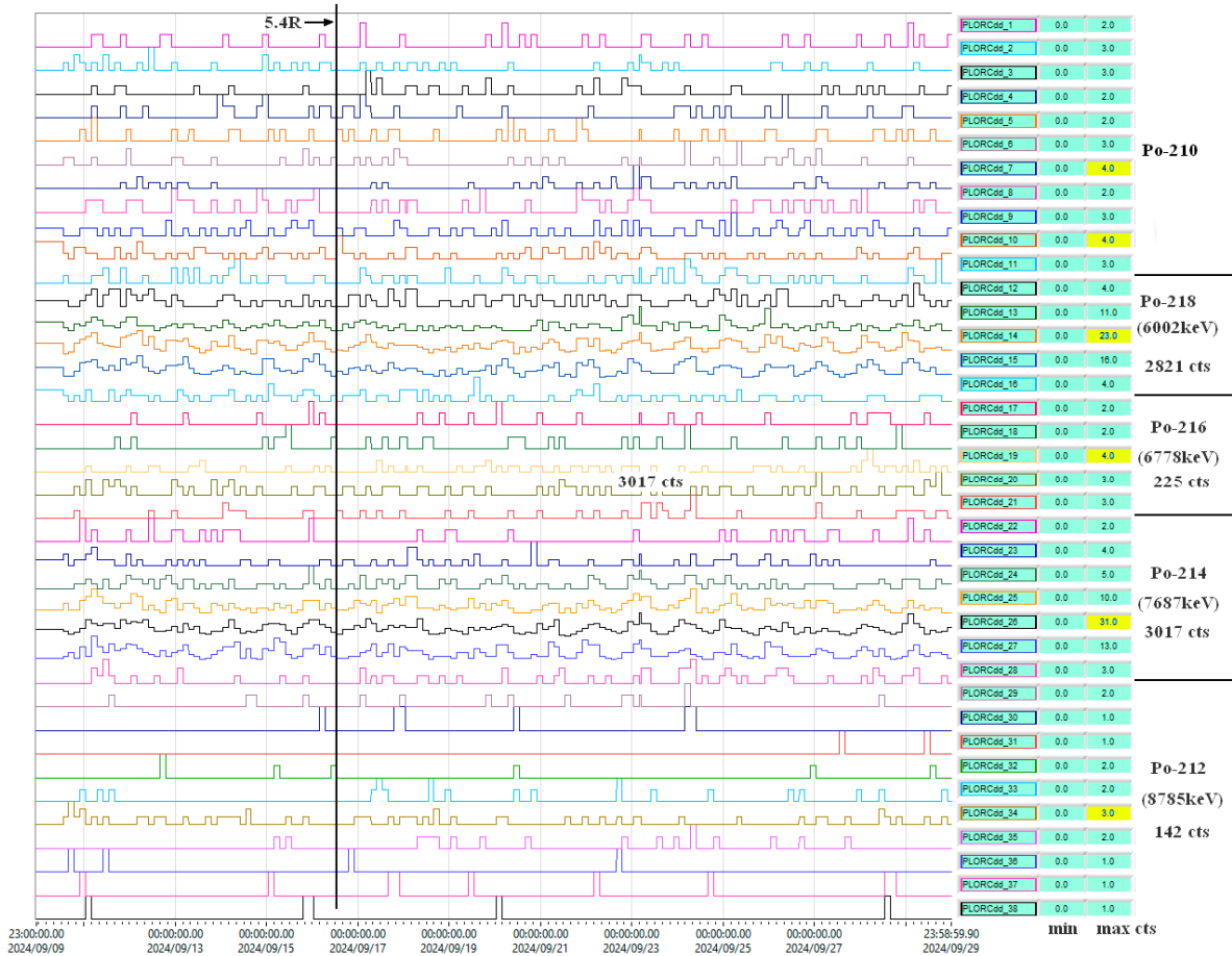
Figure 6. Determination of the Alpha spectrum from RTM1688-2 data.
