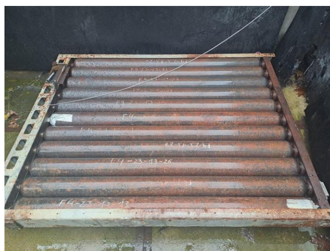
Figure 6. System after high temperature static pressure and extreme temperature cycle test.
