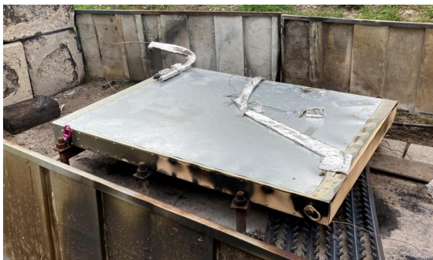
Figure 9. Condition of the test system on the test bench after the fire test.
