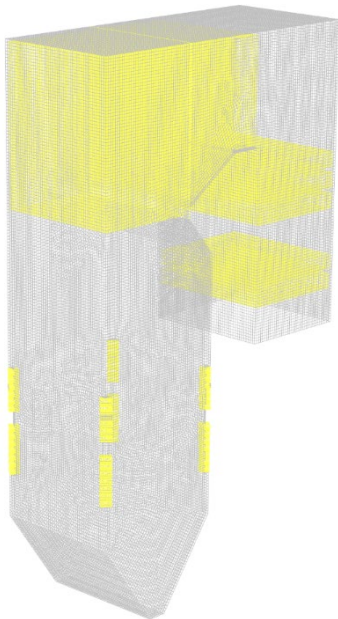
Figure 4. Mesh model of the pulverized coal boiler.
