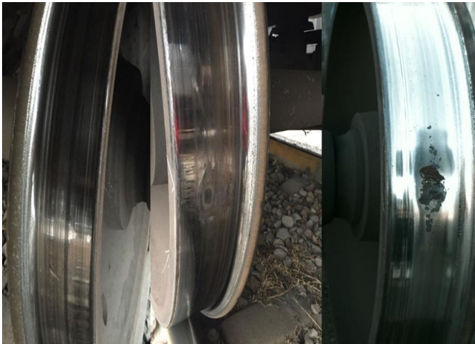
Figure 1. Three main types of defects on the wheel tread (pit, bruise, and peel).
