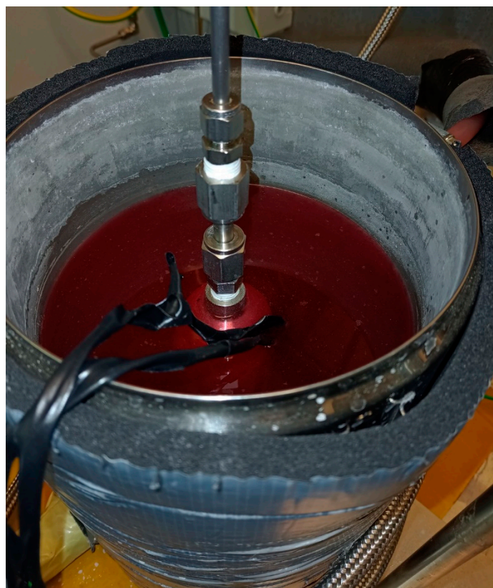
Figure A6. During the measurements, the sample cylinder is immersed in a thermobath containing a 1:1 water/glycol mixture and connected to a Julabo FL1703 temperature controller.
