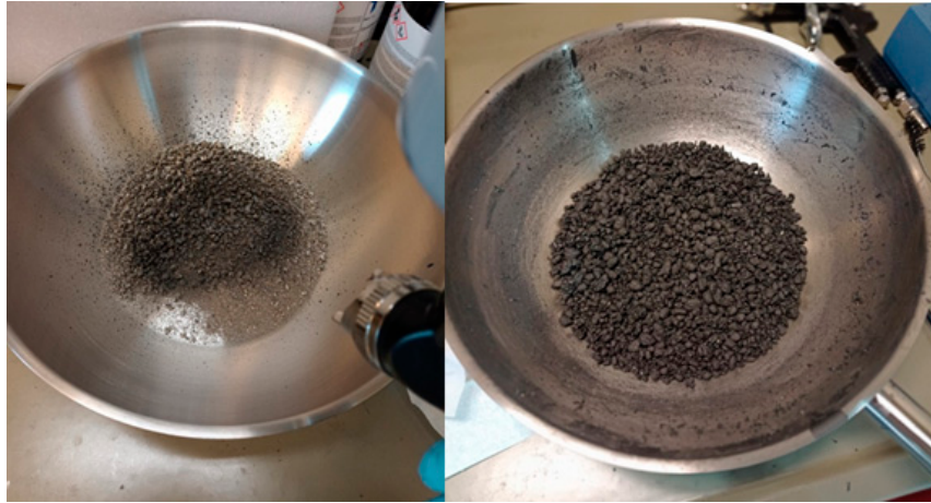
Figure A2. Comparison of the metal alloy at the beginning of the spray-coating process (left) and after the coating process is finished (right).
