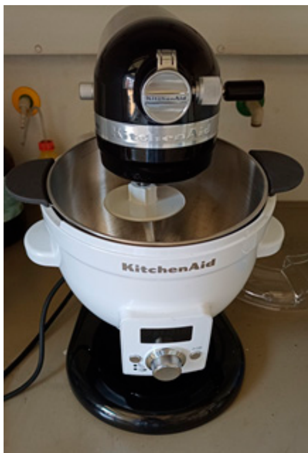
Figure A1. Image of the experimental set-up used for the larger-scale wash-coating process in a household stand mixer with a heatable bowl.
