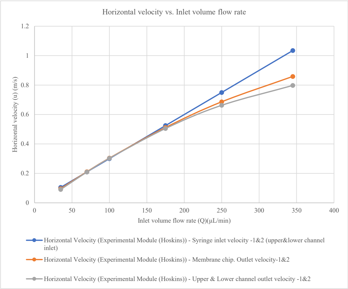
Figure 4. Horizontal velocity in experimental module (Hoskins) with constant wall permeability (module parameters in the text).
