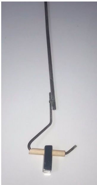
Figure 1. Coupon holder designed for pilot plant.
