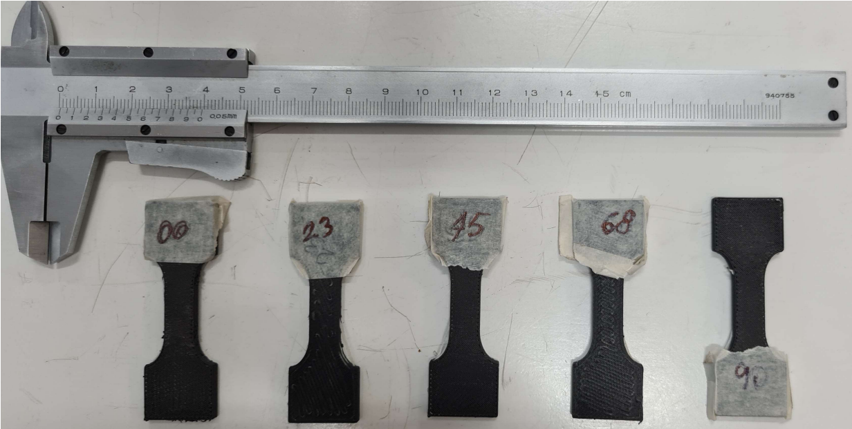
Figure 2. Example of some samples with the laminations described in Table 2, shown next to a Vernier caliper for comparison.
