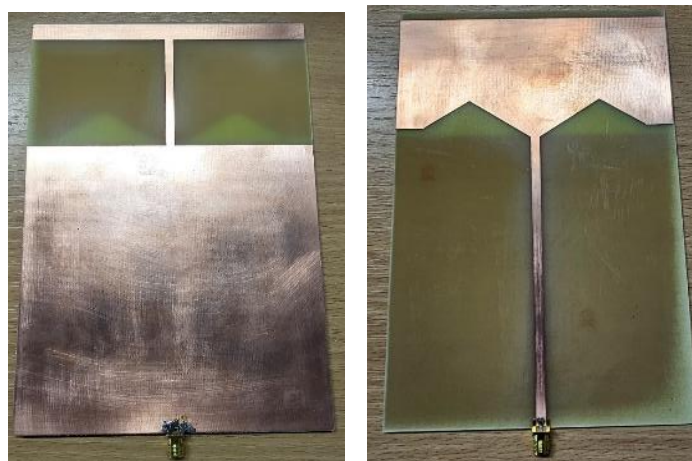
Figure 2. The view of completed DVB-T2 microstrip antenna: front view showing the radiating patch and microstrip feed line and rear view showing the ground plane.
