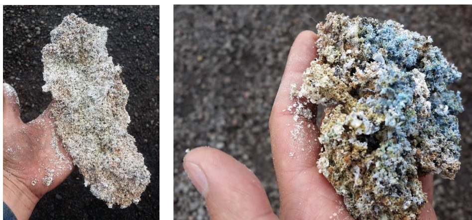
Figure 5. Large pieces of sintered ash extracted from the combustion bed of the retort burner after 60 minutes of operation, during combustion of raw coffee husks.
