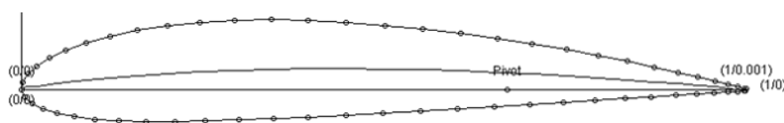
Figure 4. NACA3414 airfoil profile (JavaFoil, 2024) [27].
