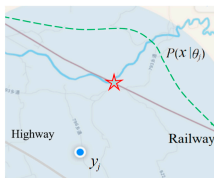
Figure 2. A GPS device's positioning with a deviation. The round point is the pointed position with a deviation, and the place with the star is the most possible.
