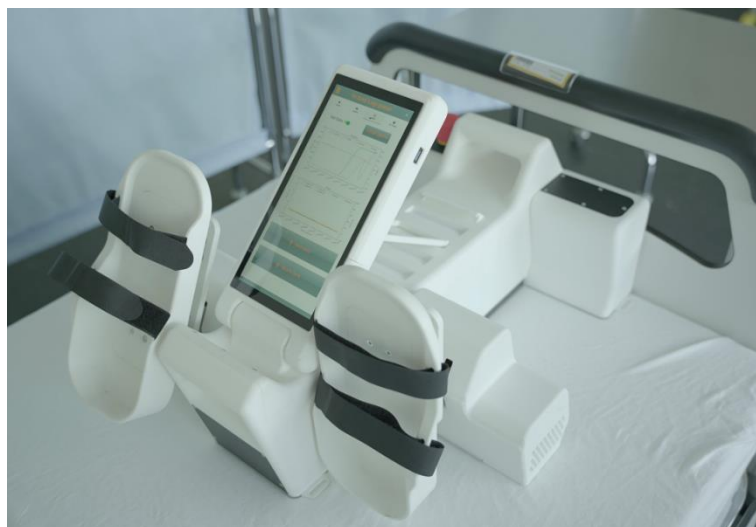
Figure 2. The prototype of the lower-limb therapy device on a medical bed.
