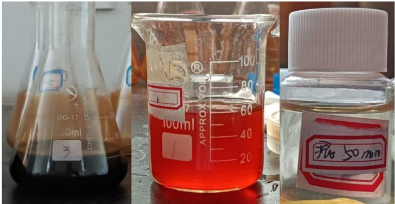
Figure 3. Comparison before and after treatment of dye wastewater by combined process of iron carbon micro-electrolysis + coagulation sedimentation. (The left: the raw water, The middle: the supernatant of iron-carbon micro-electrolysis experiment, The right: the best coagulation sedimentation effluent).
