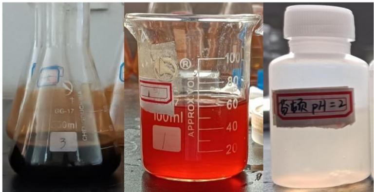
Figure 4. Comparison before and after treatment of dye wastewater by combined process of iron carbon microelectrolysis + Fenton oxidation. (The left-the raw water, The middle-the supernatant of carbon micro-electrolysis experiment, The right-the out water of Fenton oxidation).
