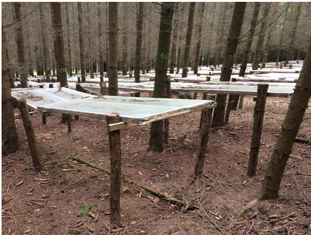
Figure.1 1. The treated plot where 60% of the soil surface was covered with PE foil.
